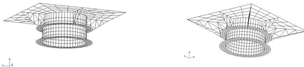
Figure 3 – Stiffened lower panels of models MST1 (left) and MST2 (right)
